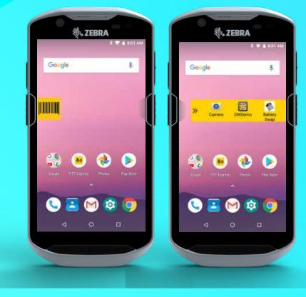
Enables users to place a customizable on-screen soft button on either side of the display
